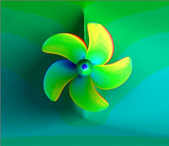
Fig.11: Rear view of instantaneous computed dynamic pressure distribution on hull and propeller
